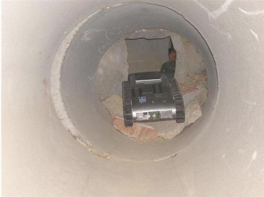
Fig. 65: Robot going through a wrecked pipe to find a person
