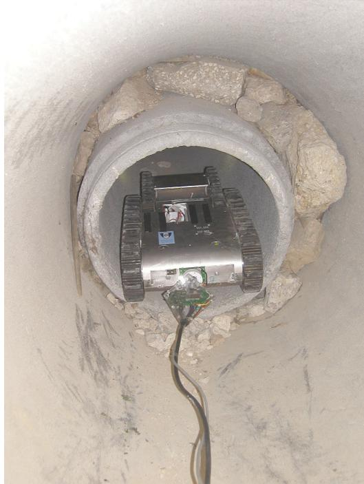
**Fig. 69: Raposa on Empty water pipe**
