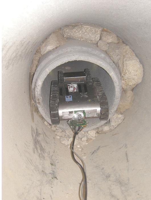
**Fig. 69: Raposa on Empty water pipe**
