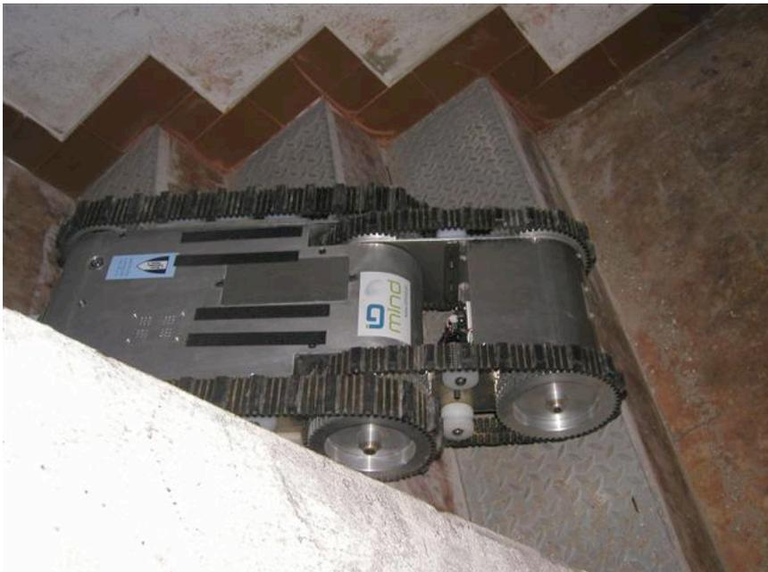
Fig. 66: Robot going downwards through stairs
