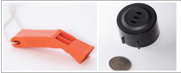
Figure 2.11: (a) The safety whistle used in the experiment (commonly available in outdoor shops). It features two chambers, and emits two closely spaced, superimposed frequencies between 2kHz and 2.1 kHz. (b) A hand-held piezo alarm that emits a single frequency of 3.8 kHz.
