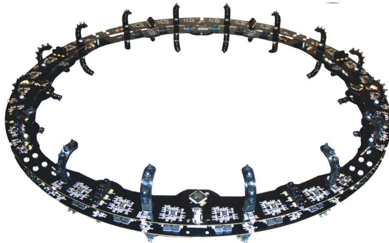
Figure 1.6: Sensor suit proposed by [Roberts et al., 2009] for an on-board relative positioning system for an indoor flying team of robots. This sensor suit weights  $\approx 400$  grams and consists of 160 IR transmitters and 48 photo diodes and is capable of providing accurate 3D range and bearing inside a range of 10 meters.
