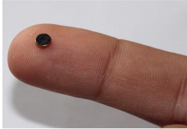
Figure 1.4: Picture of a commercially available omnidirectional microphone sensor used in some part of this work, purchased at a price of around 1 Euro, that has a radius of 2mm and a weight of 0.04g
