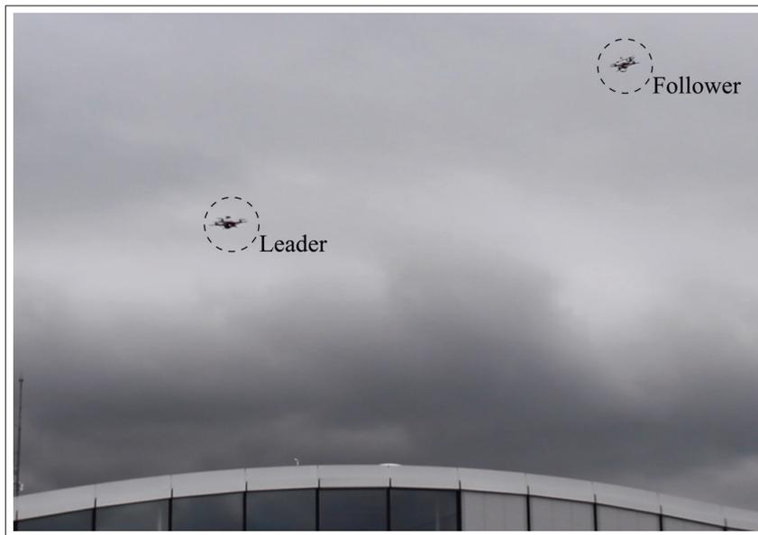
Figure 3.26: Photo showing an instance of the audio-based leader-follower experiments involving two rotorcraft MAVs, where a fully autonomous follower MAV used the on-board active relative bearing measurement system to reactively follow a teleoperated chirping leader robot. Videos can be found at <http://lis.epfl.ch/ABSMVA>
