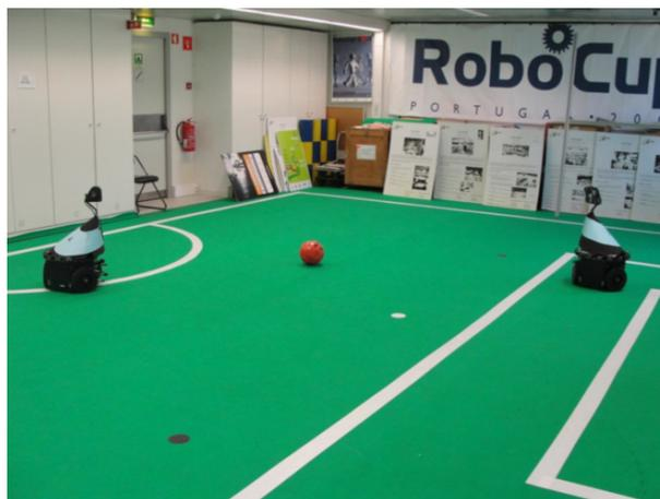
Figure 4.5: Real robot view for one of the layout locations: the robot on the left is the robot that informs the correct ball position to the other, while the robot on the right is the kidnapped robot which uses that information, in location 4 of Figure 4.4.
